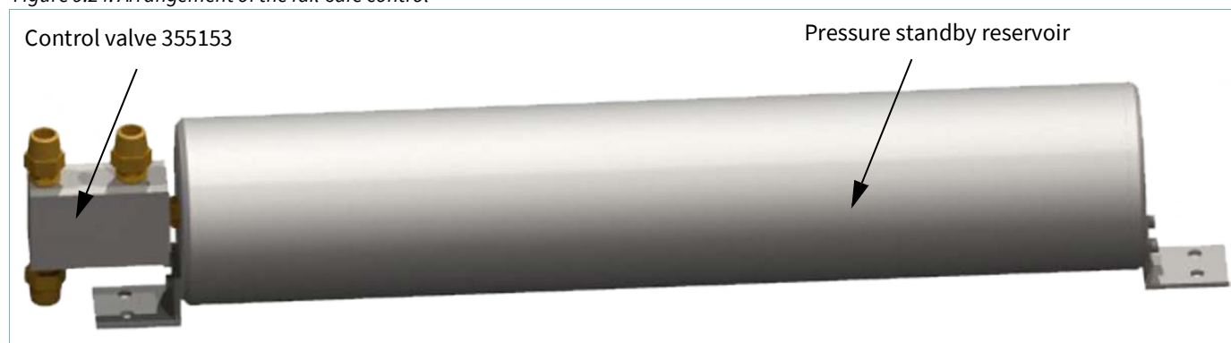
Figure 9.24: Arrangement of the fail-safe control
